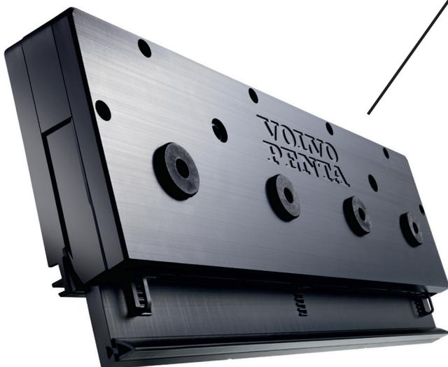
The compact interceptor blades require minimal maintenance thanks to the composite materials. The blades have an automatic, self-cleaning function and a full stroke of 50 mm.
